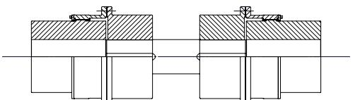
FLOATING SHAFT MILL-MOTOR
