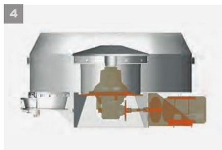
gearbox and driven by it is a hydraulic gear pump which constantly cycles the oil. Gearbox and discharge gate(s) use the same oil for less maintenance. This oil also supplies the pressure to operate the discharge gate(s).
