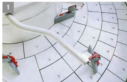
**2** | Central lubrication for the mixing arm bushings is available. Depending on the application, mixing paddles, wall scrapers, and mixing arm wear guards made of various abrasion-resistant materials are available. These include cast-iron W4, with complete tungsten-carbide surface, polyurethane-elastomere (PU), SPIKE cast-iron, nickel-free special casting, etc.
