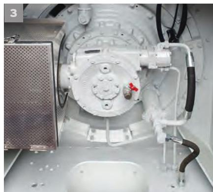
**3** | The centrally located planetary gearbox is driven by a 3-phase TEFC motor which is flangemounted directly to the gearbox, in the case of pan-type mixers THZ 375 to THZ 1125.
