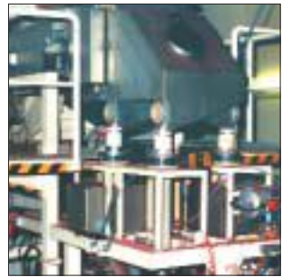
Figure 45 SR 18/6-IV quadruple-deck screening machine with downstream metal detector
