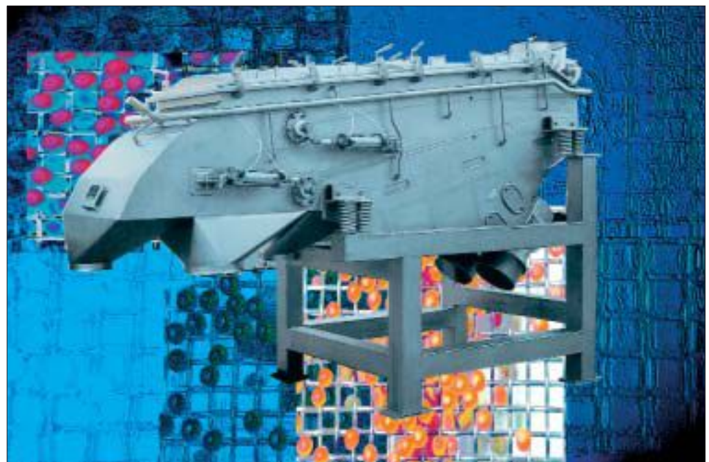
Figure 2 SR 25/10-II vibratory screening machine with 2 screen decks, pneumatic screen-tensioning device and CIP mechanism for screening milk powder
