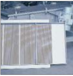
Figure 23 The perforated-plate screen insert has no gaps or sharp-edged corners
