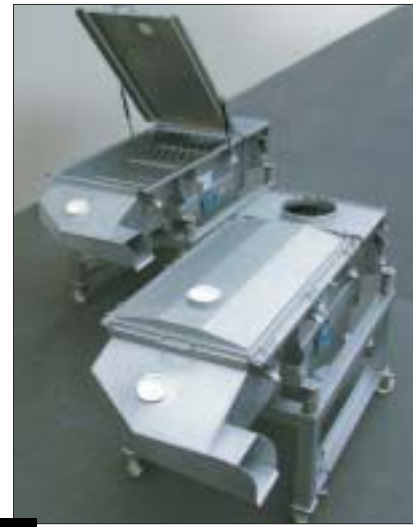
Figure 17 Quick-action clamps and gas springs provide optimum operating convenience
