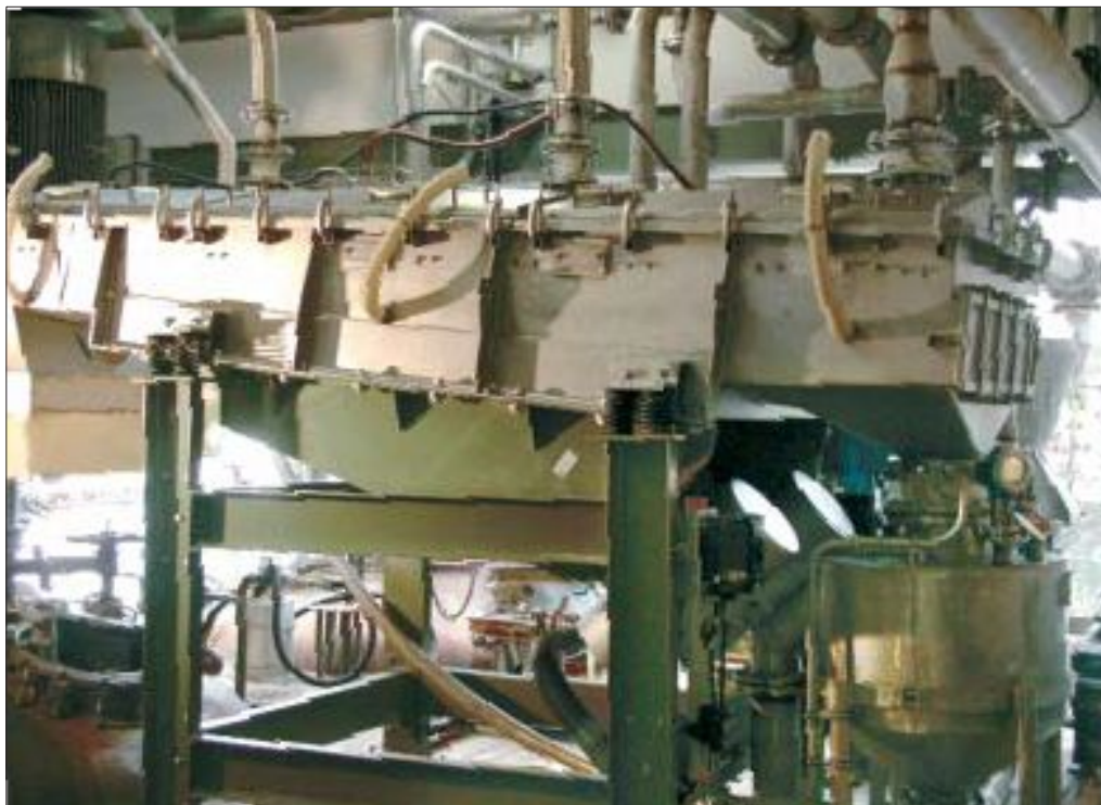
Figure 43 SR 30/10-III triple-deck screening trough conveyor with pneumatic screen-tensioning device for the screen linings
