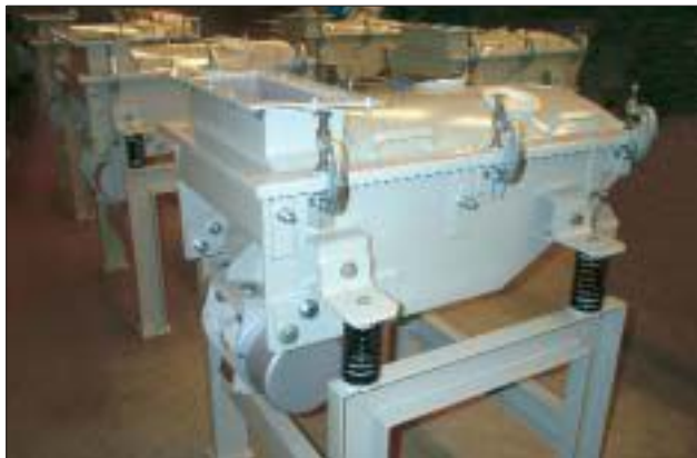
Figure 37 SLUG 8/5 screening machines
