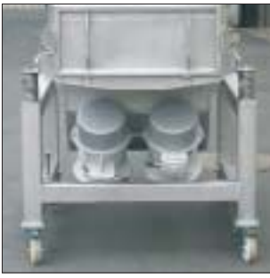
Figure 18 The robust twin motor vibrator unit produces directional vibration and has infinitely variable unbalance
