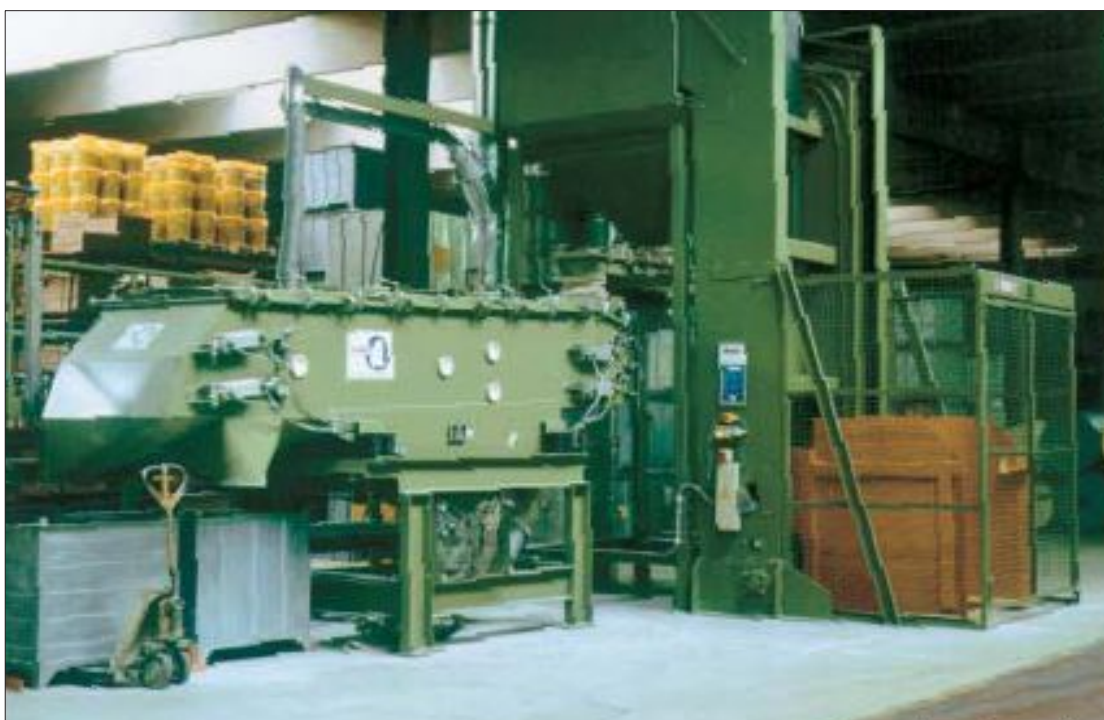
Figure 41 SR 36/10-II twin-deck vibratory screening machine with coating station in a rubber factory
