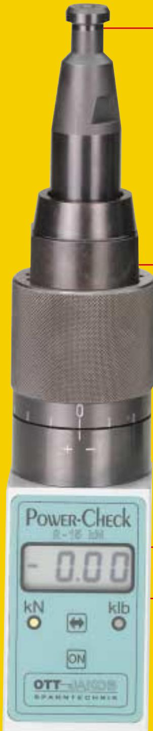
All SK work holders from SK30 to SK60 (DIN/ISO/ANSI) and all HSK work holders according to DIN 69893 (HSK-A 32/B 40 to HSK-A 125/B 160) can be used.
