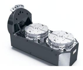
**One-arm rotary tilt tables** compact design for simple table loading and good access during the machining process
