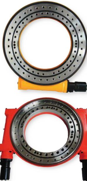
The space saving all-in-one solution for different kind of applications. The reliable slew drives from RODRIGUEZ consists of a geared slewing bearing and suitable worm or pinion in a compact housing. Moreover, all slew drives can be delivered including a mating drive motor in electric or hydraulic version.
