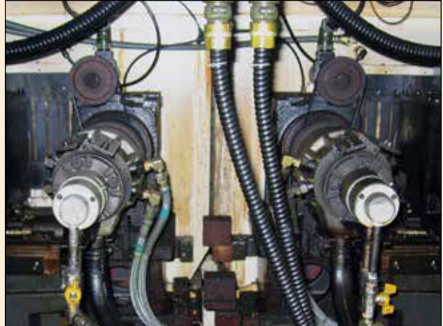
DEUBLIN 2-passage Unions on CNC Turning Center
