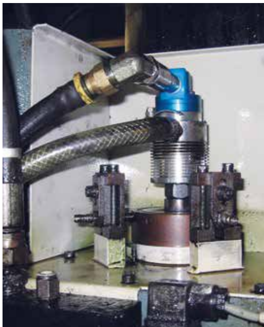
DEUBLIN 1109 on vertical machining center
