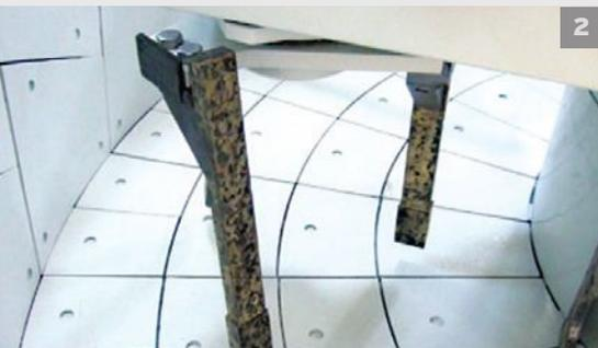
TEKA pan-type mixers THZ are also available with mechanical and hydraulic agitators. Mechanical agitators have a fixed rotation speed. The hydraulic agitators allow for infinitely variable rotation speeds. [www.precise-rotation.ru](http://www.precise-rotation.ru)
