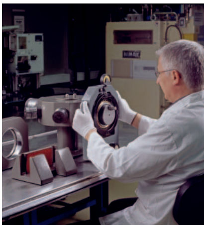
11: Position of enveloping circle gauge
