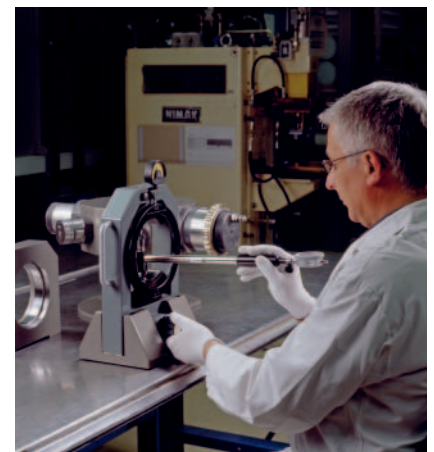
10: Transfer of the raceway diameter to the enveloping circle gauge
