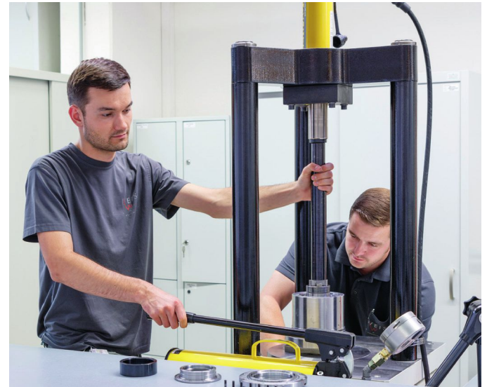
Careful disassembly of the spindle unit ensures cost-effective corrective maintenance
